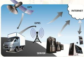
How does a GPS based tracker work?
